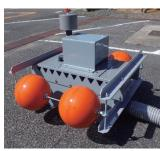
Horizontally arranged oxygen dissolution devices supply oxygen from a shallow depth of about 0.2m below the surface, covering various water depths.
