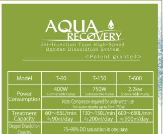
For Aquaculture tank and Aeration tank in wastwater treatment facility
